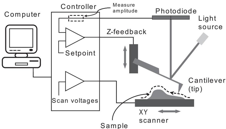
**FIGURE 2.** Schematic of the operation of the AFM. To obtain an image, a cantilever is scanned over the sample surface. A laser beam is deflected off the back of the cantilever, and changes in deflection are monitored with a photodiode detector. Reprinted with permission from Asylum Research (Santa Barbara, CA).
